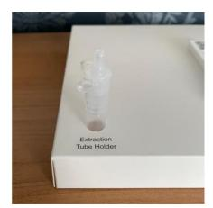
7.) Close the lid on the extraction tube and put it in the tube holder.
