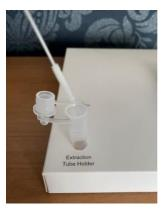
15.) Put the soft end of the swab into the extraction tube so that it is in the liquid at the bottom
